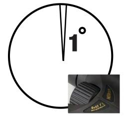
AOV, like a circle is made up of  $360^{\circ}$ ,  $1^{\circ}$  is = 15.97m at 914.4m (52.4 ft at 1000 yards)
